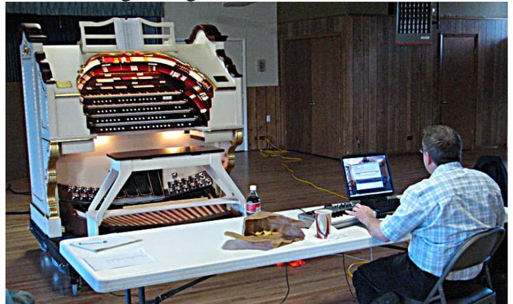
Using his laptop computer and the Allen organ DOVE (Dealer's Organ Voicing Editor) software, Walt meticulously adjusted every note of every stop on the instrument. He modified sound sample positions, adjusted individual note volumes and used digital filters to modify "pipe" voices.
